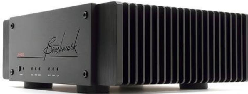
A stereo amplifier running in bridged mono mode will produce twice the voltage and can produce up to four times the power into a given load. The Benchmark AHB2 power amplifier is about 6 dB louder when running in bridged mono mode.
